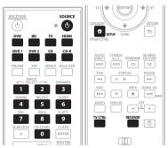
**1** While pressing the RECEIVER button, press SETUP. The indicator on the remote control blinks.
